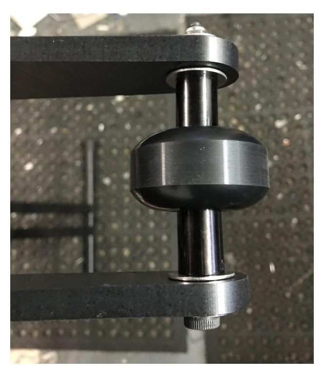
Put a washer on the wheel shaft then through the left side bar, then another washer, nylon spacer, wheel, spacer, washer, then another washer M6x25 and then M6x10 washer and finish with a nyloc nut on the other side, tighten up and you have completed the installation.
