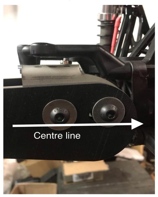
Take notes how the M8 bolts are fitted above, you have separate adjustments to change the bars for no wheelie to a high wheelie, the left hole as pictured above is not an adjustment this is fixed and secures the bars to the bracket only.
