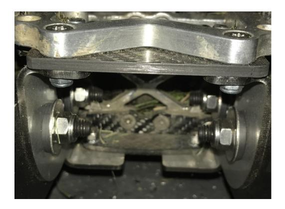
Now fit this brace with M4x30 countersunk screws and M5x12 button heads, again fit loosely at this point to make sure the brackets have all the bolts started first.
