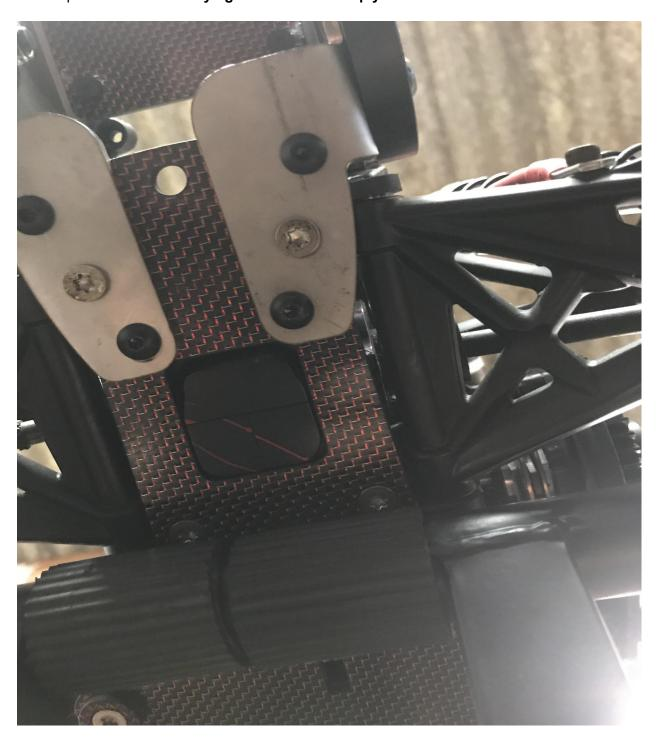
Now fit the carbon reinforcing brace, this fits in two different ways depending on what upper rear bulkhead you have be it stock plastic or aftermarket alloy, if you have the stock plastic then the carbon plate fits as pictured with the carbon plate under the bracket.
