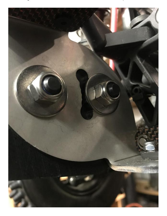
Now tighten these bolts right up to secure the bar fully once your happy with the wheelie bar angle you have chosen.
