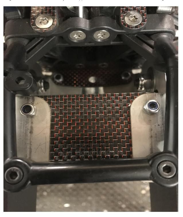
Now you can assemble the bars to the brackets the holes need to be fitted so they are above the centre line of the bar, see Picture for guidance.
